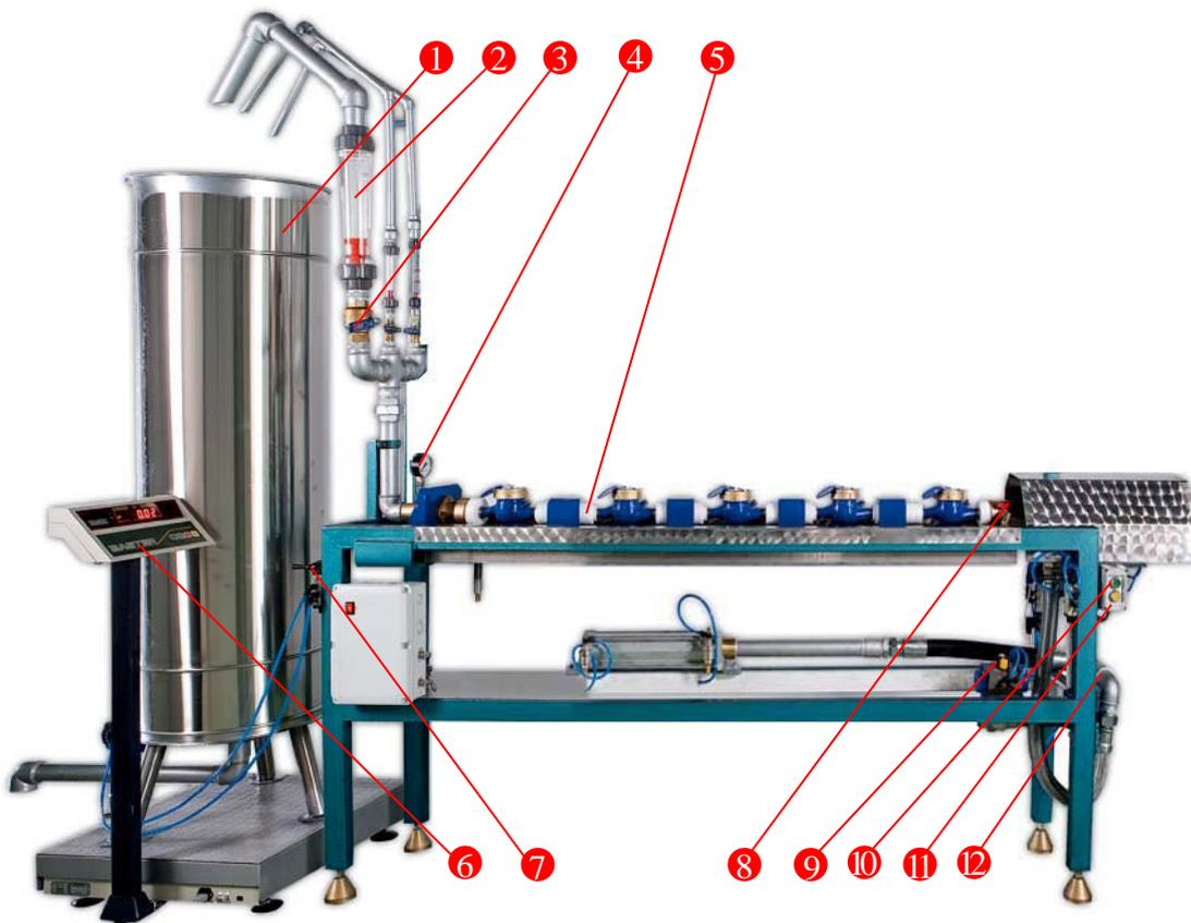
The test bench main frame is consist of, steel skeleton and stainless sheet metal combination. Steel skeleton is plated with wet epoxy paint. There is a pneumatic regulator for providing constant air pressure. Space connecting pipes is made of P.O.M. and protected against shock and bending.
