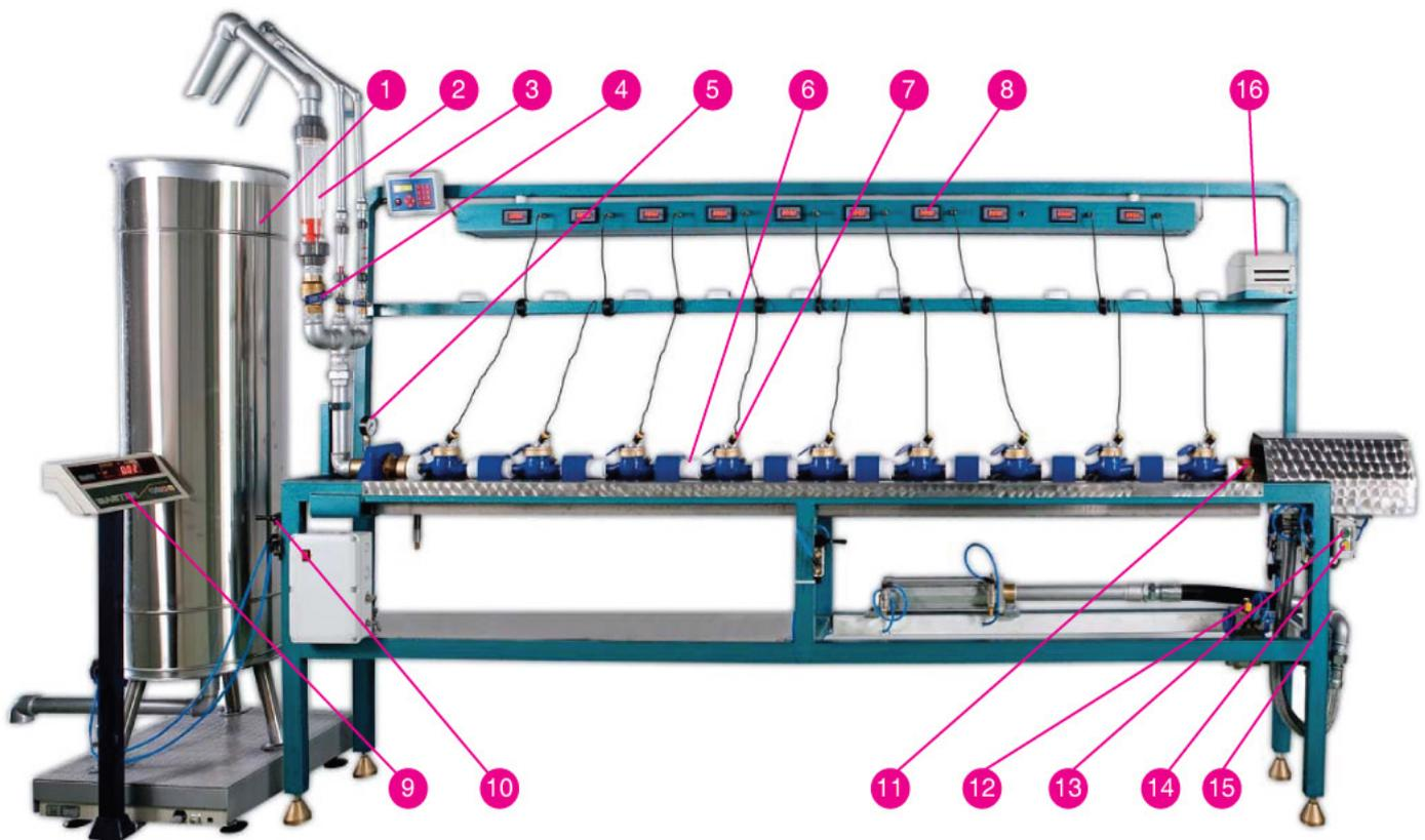
The test bench main frame is consist of, steel skeleton and stainless sheet metal combination. Steel skeleton is plated with wet epoxy paint. There is a pneumatic regulator for providing constant air pressure. Space connecting pipes is made of P.O.M. and protected against shock and bending.
