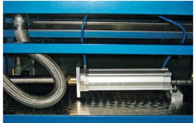
Push the stick until the pressure reaches your test pressure. Then leave the stick and wait the time of test with static pressure. When the test time is okay, push the stick to left and release the pressure. Close pneumatic water inlet valve before opening the system, and also open the system pressure release valve(pic1/18) and see on the system manometer there is no pressure.
